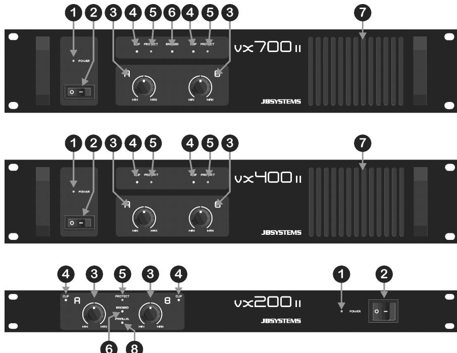
1. **POWER LED:** This blue led is on when you turn the amplifier on using switch(2).
