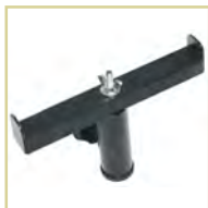
SST-20 Code : H8262 For PT20-150 truss only Bar length: 21 cm Section of the bar: 30 x 20 mm Internal diameter of the stand adaptor: 28 mm M8 screw for fastening the truss Finish: matte black epoxy paint Weight: 0.40 Kg
