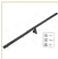
BRE-120 Code : H8256 Internal diameter of the stand adaptor: 28 mm Bar length: 1.20 m Bar section: 30 x 30 mm Number of holes: 4 Materials: Steel and ABS for the knob Finish: matte black epoxy paint Net weight: 1.6 Kg
