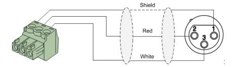
For unbalanced signal input connections
