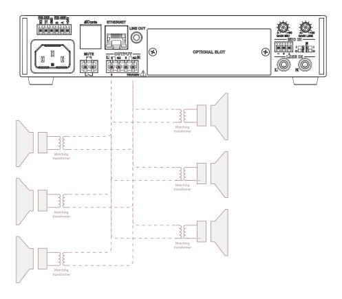
Depending on the chosen connection method (low impedance or constant voltage), the output configuration setup shall be configured accordingly.
