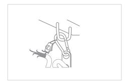
Connect the speaker. The correct power tapping is chosen by connecting the appropriate conductors to the wires coming from the amplifier. A description of the power tap selection is shown on the sticker on top of the loudspeaker or as follows:
