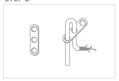
Slide the ceiling cover cap over the connection wire and put the connection cable through the bottom hole of the included plastic wire holder as shown in the drawing. Feed the cable through until the required cable length for suspending is reached. Then pull the cable through the second hole (middle one) until it is tight.
