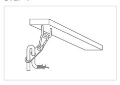
Hang the speaker to the provided point on the ceiling and fix it by suspending the plastic wire holder to it using the included snap hook.
