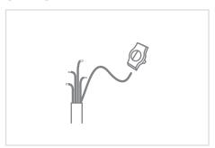
Cut the excess length of the cable to the desired length for reaching the connection box, and remove the outer jacket for about 10 centimeters.
