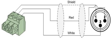
For unbalanced line output connections:
